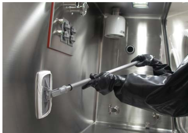
Figure 1. Isolator cleaning tool in use (Photo courtesy of Getinge, LaCalthene)
